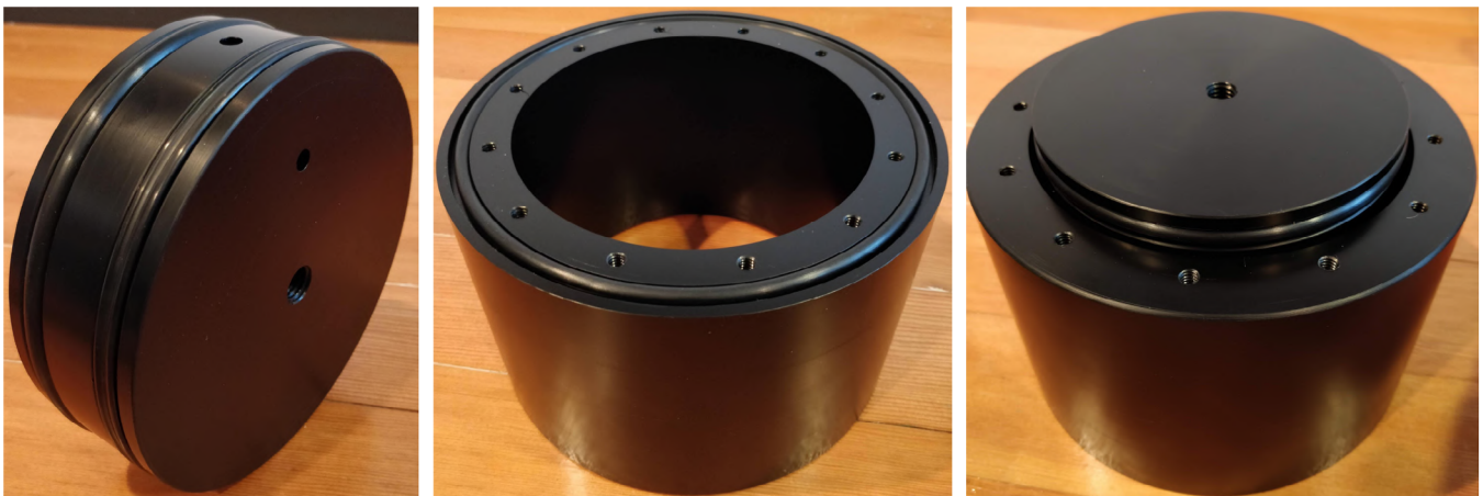
FIG. 5. Left: Piston with dual O-rings; Center: Cylinder with O-ring to seal against base plate; Right: Piston in Cylinder. Threaded blind hole in piston to couple lung motion is visible.
