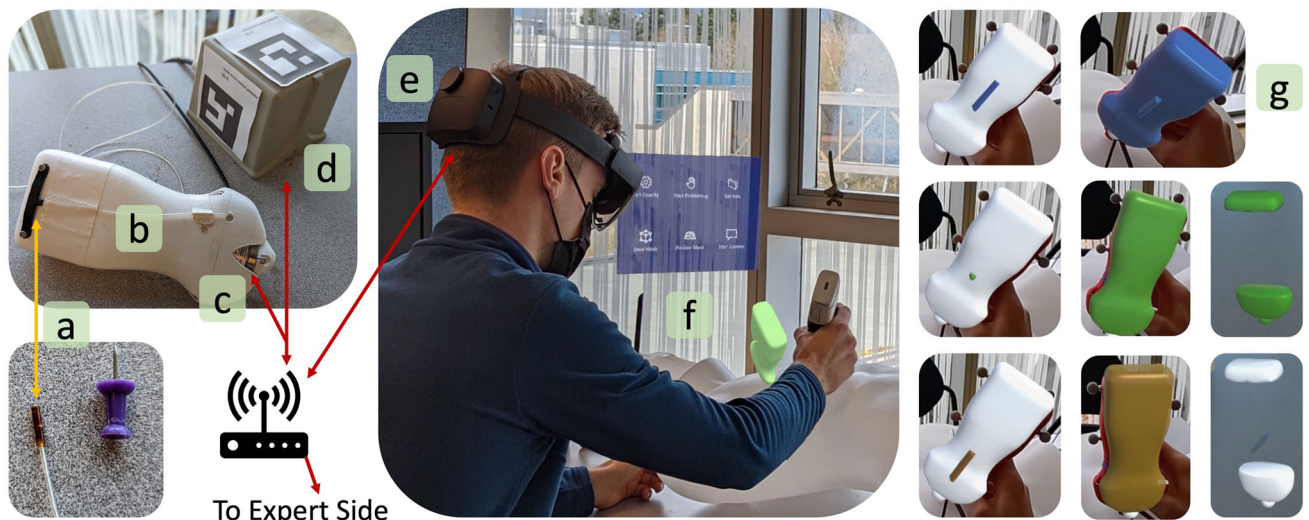
Fig. 1 System overview: a electromagnetic tracker (on device and separate, with thumb tack for scale); b dummy US probe; c force sensor; d electromagnetic sensing transmitter with ArUco markers for registra-
