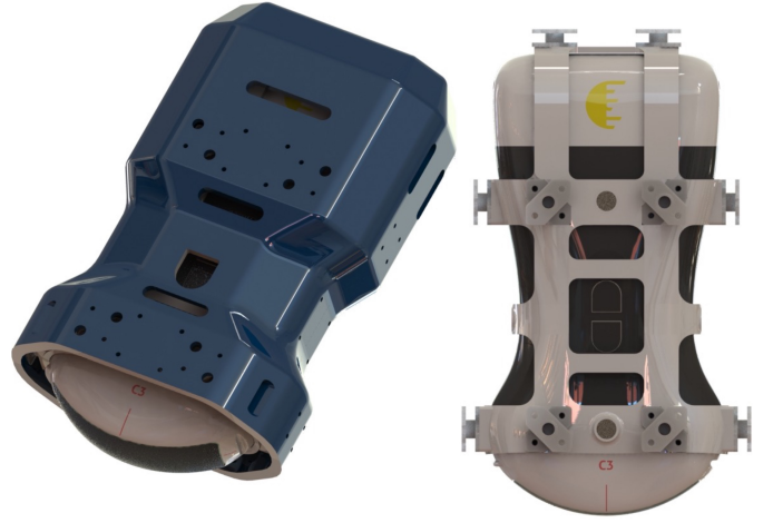
Fig. 1. Design and integration of 6-DOF force sensor onto a C3HD 3 ultrasound probe (Clarius, Vancouver, BC), with inner scaffold, compliant suspension, outer shell, and electrical integration.
