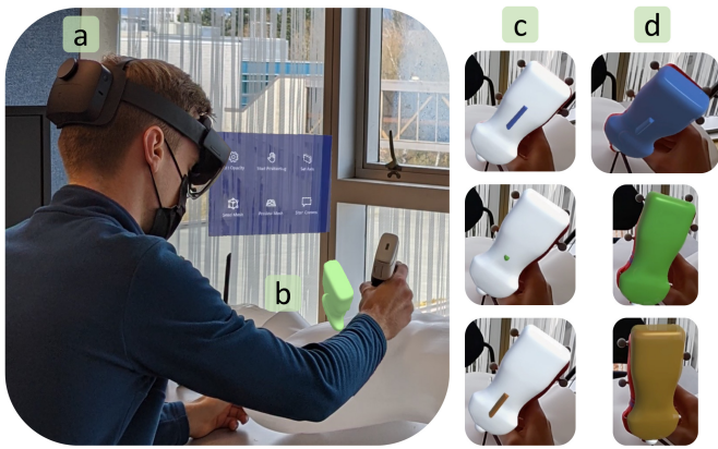
Fig. 3. Follower side showing the follower wearing a HoloLens 2 (a), the holographic user interface (b), and the different force rendering schemes: Error-bar (c), and Color (d).
