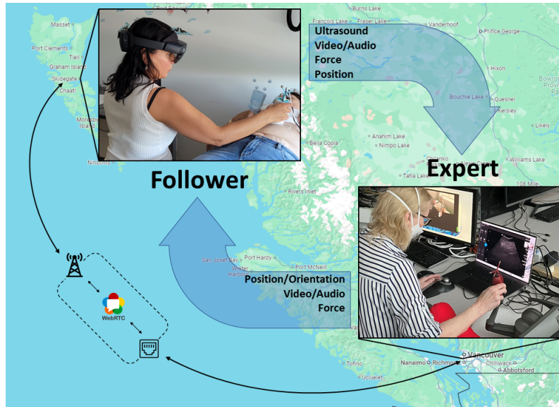
Figure 1: High-level system diagram illustrating the mixed reality teleultrasound system being used over a large distance.
