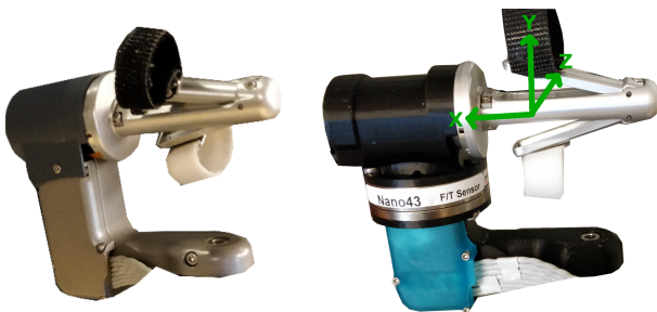
Fig. 1. The original (left) and instrumented MTM (right), overlaid with the local coordinate system also seen in Fig. 3
