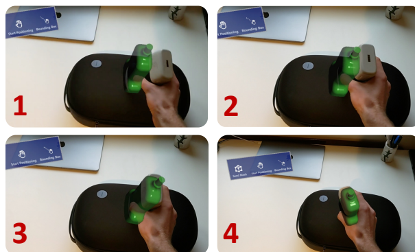
Fig. 1 The teleoperation concept. Frames 1-3: follower matches the virtual probe precisely, starting in a random pose. Frame 4: the expert moves the virtual probe, and the real one quickly tracks the motion.
