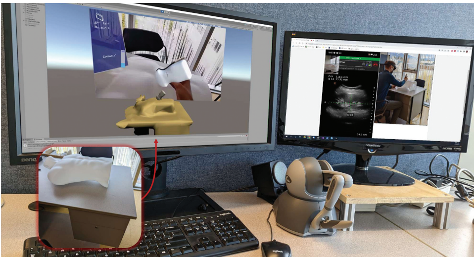
Figure 4. Expert Workstation: the Phantom Omni haptic controller (front center) is used to input pose and force and provide haptic feedback. The virtual probe relative to the patient mesh is visualized on the left monitor along with the live MR capture. A cutaway on the bottom left shows the real environment which is recreated closely by the mesh. Fig. 3 shows further MR captures. The Clarius live ultrasound images and video call are shown on the right monitor. Note, no actual ultrasound image was captured of the dummy, so the displayed image is a screenshot from a patient test, pasted here to portray the complete expert side.
