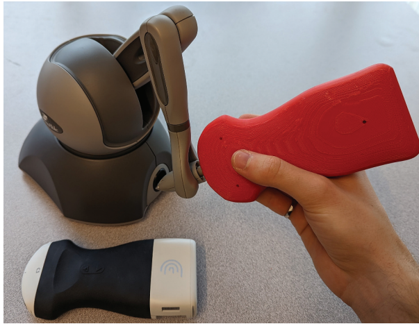
Figure 9. Ultrasound probe-shaped end effector mounted on haptic device for pose following tests.
