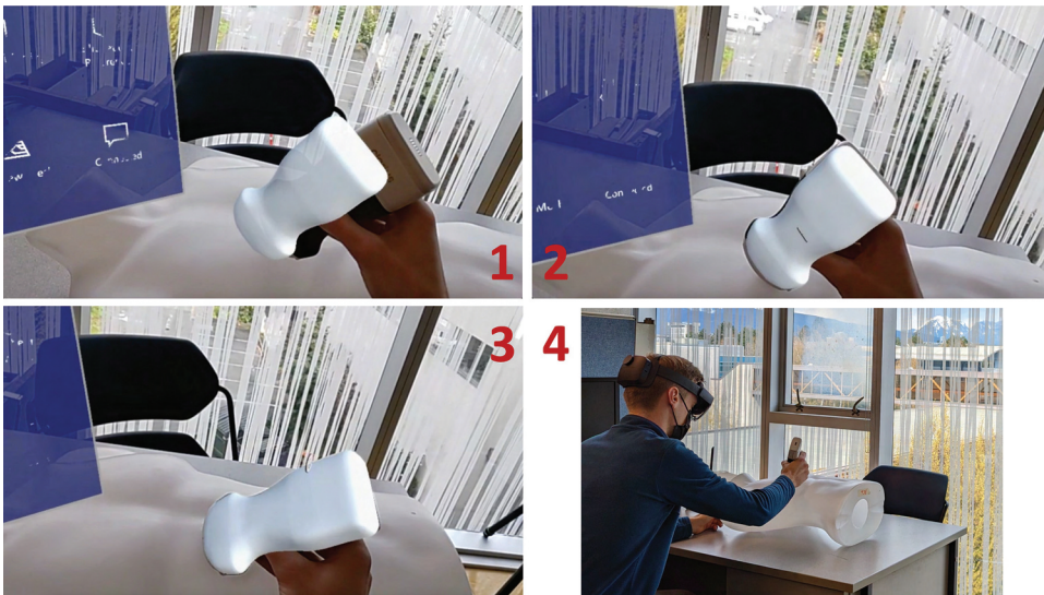
Figure 3. Follower-Side Interface and Teleoperation: The follower sees the virtual transducer and a control menu. In frames 1-2 the follower starts in a random position and matches the virtual probe pose precisely within < 0.5 sec, before the probe pose changes and is immediately matched by the follower again in frame 3. Frame 4 shows the follower during this test. An image of the expert side during the creation of this sequence is shown in Fig. 4. The full test is available as a video - see Supplementary material
