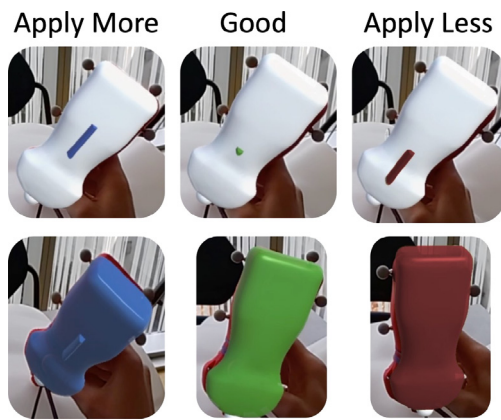
Fig. 6. Color and error-bar force rendering schemes, showing the desired follower action for each rendering. Note, the color and bar length vary continuously and linearly between the shown states.
