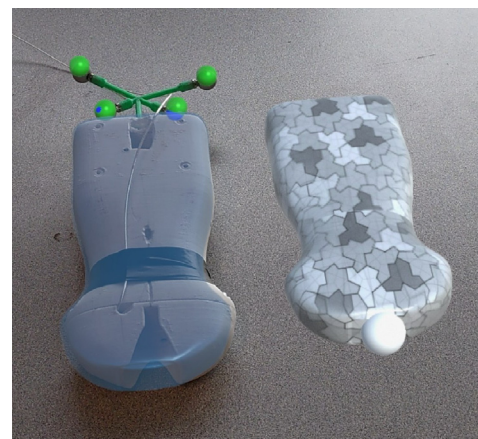
Fig. 5. MR Capture from HoloLens 2 of (Left) the dummy ultrasound probe with IR markers showing successful pose tracking. The green spheres are the measured marker positions while the blue ones are the output of the unscented Kalman filter, and the blue virtual probe shows the resultant calculated pose. This preview can be disabled during actual operation. And (Right) the virtual ultrasound probe controlled by the expert, with patterns for better contrast and depth perception. These can also be seen in videos in Supplementary Material.
